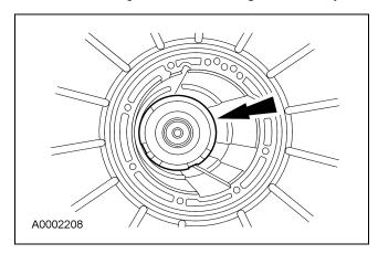
31. **NOTE:** The No. 13 bearing must be properly seated in the forward planet assembly so the sun gear can be installed correctly.
